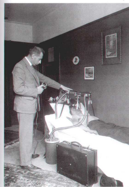
Fig. 67 The transportable Metalix Junior D workstation. This system was also useful for examining bed patients.
